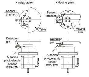
Install an additional sensor to detect home position and to ensure motor's positioning, number of rotation and its speed.
