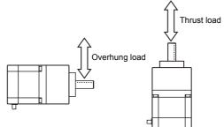
Refer to the table below for allowable shaft overhung load / thrust load.
