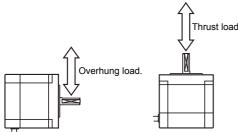
Refer to the table below for allowable shaft overhung load / thrust load.
