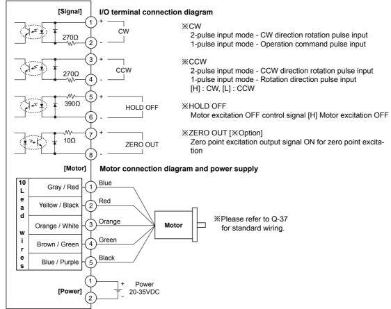
**Note)** Add external resistance when power for pulse from the external of the unit exceeds +5V. (Input current:10 to 20mA) **Note)** 2/3-axis use power supply in common and input/output terminals are proportional to the number of axises of mode.
