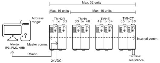
※Internal communication: Receive/Send data between TMH2/4 and TMHA/E/CT External communication: Communicate
