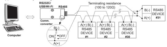
XIt is recommended to use Autonics communication converter; SCM-WF48 (Wi-Fi to RS485·USB wireless communication converter, sold separately), SCM-US48I (USB to RS485 converter, sold separately), SCM-38I (RS232C to RS485 converter, sold separately).
