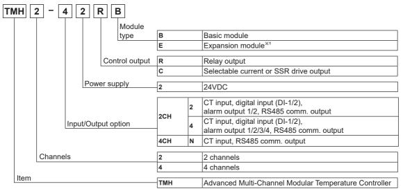
×1: Since the expansion module is not supplied with power/comm. terminal. Order it with the basic module.
